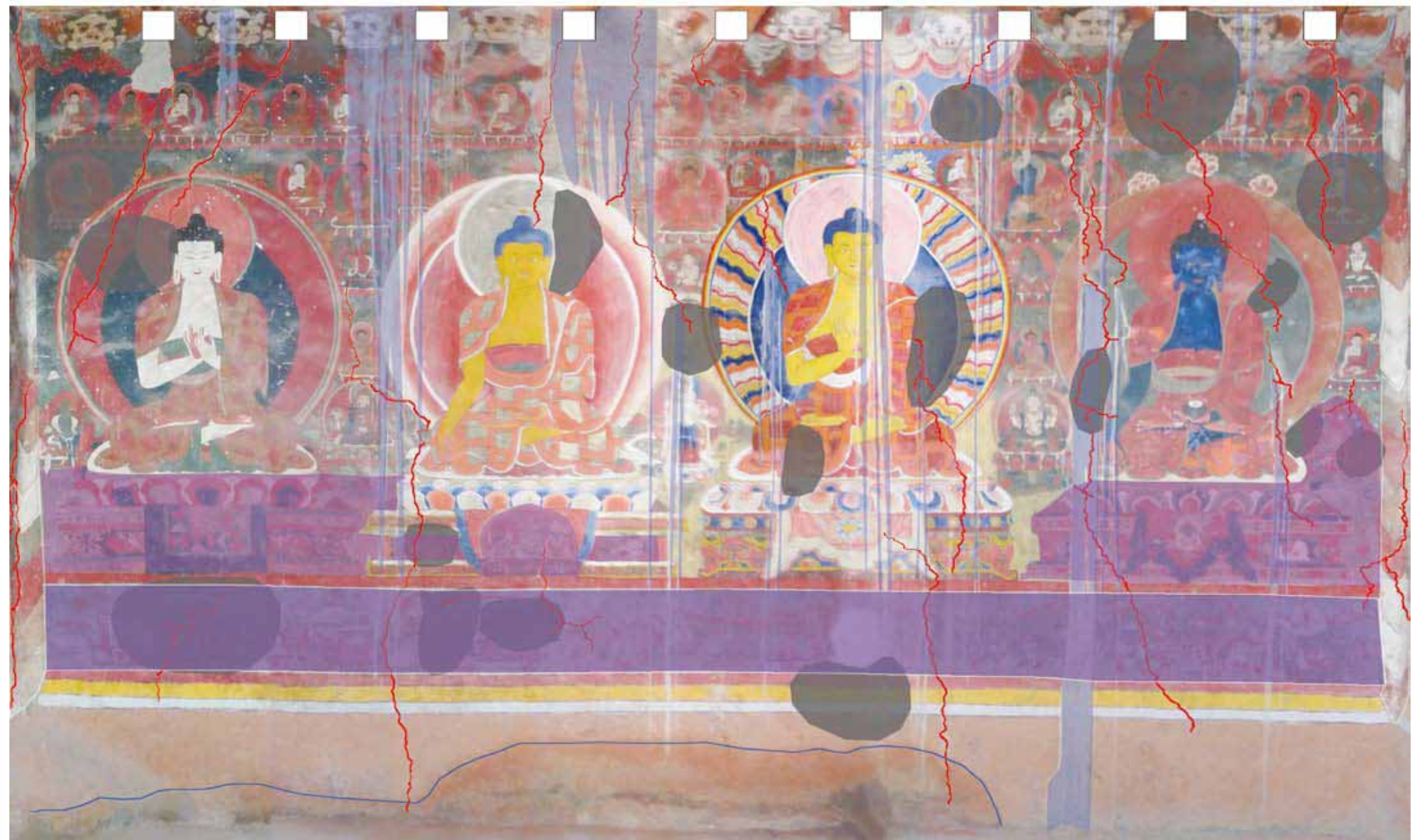
Map.15. The Lhakhang Gongma Southeast wall showing voids, cracks, washouts and drips, a water horizon, flaking and thinned painted surfaces
