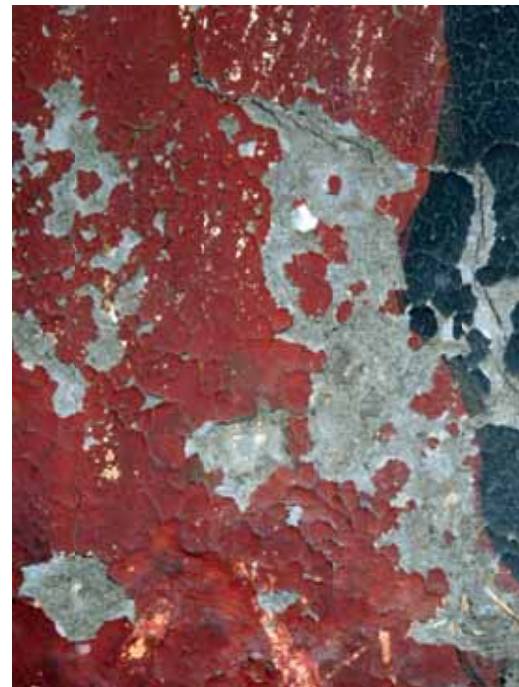
Fig.10. Detail of losses and flaking areas
